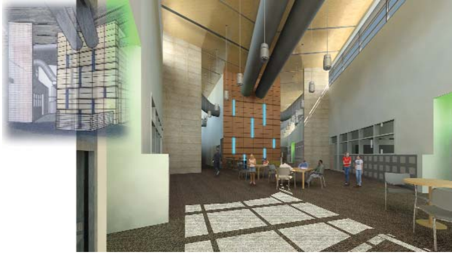
Renton Shared Learning: In the shared learning space LED accent lighting changes color based on the total energy used in the school. Separate accent lighting at classroom entries change color based on energy used in each building zone.
