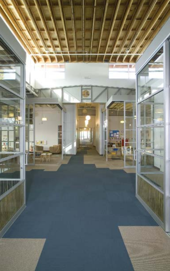
Mother's Club Interior: Interior view of the Mother's Club Family Learning Center central play atrium. Transparency combined with high bay clerestories bring natural daylight into interior spaces and foster a sense of community within the building.
