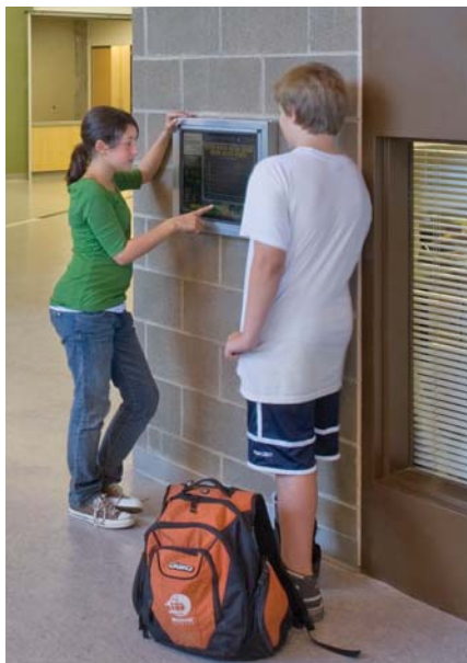
Pioneer MS Touchscreen: The touchscreen device provides easy access to current events, energy metering data (water, gas electricity) and weather data. Teachers and students can utilize this technology to explore responsible energy usage within the building.
